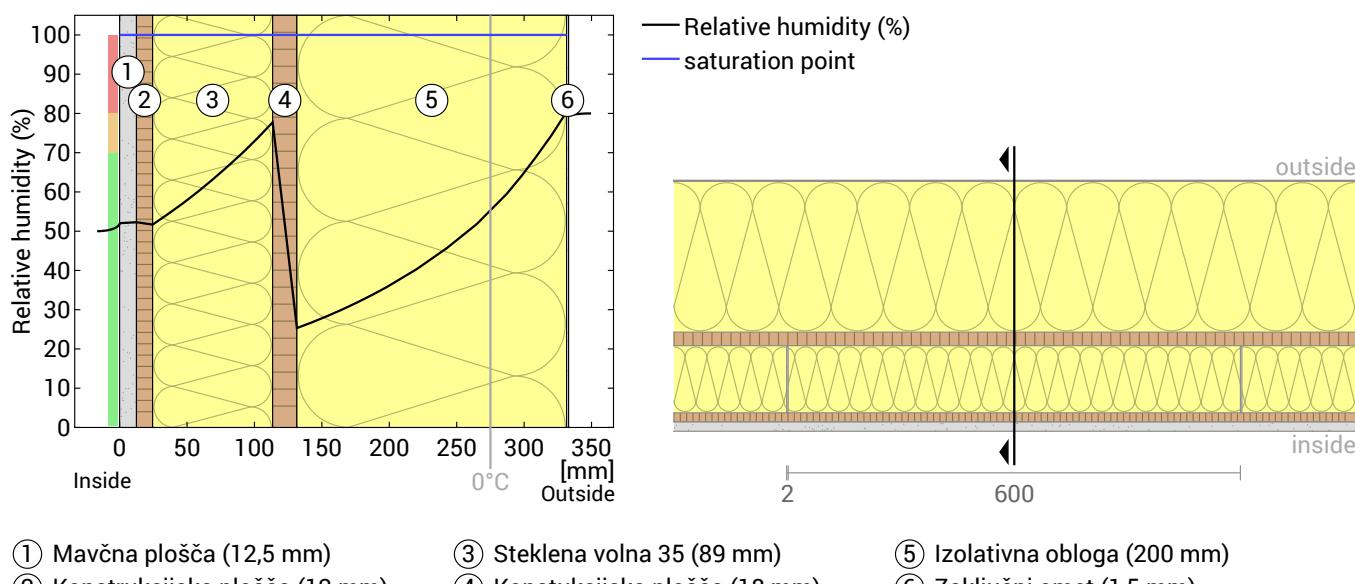
Notes: Calculation using the Ubakus 2D-FE method. Convection and the capillarity of the building materials
