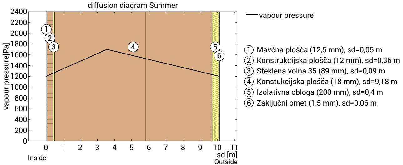
Condensate-free component: The maximum possible evaporation mass for the drying reserve is calculated. Consider the level that has the lowest evaporation potential in the dew period, at  $sd=3,56 \text{ m}$ , within layer Konstrukcijska plošča:
